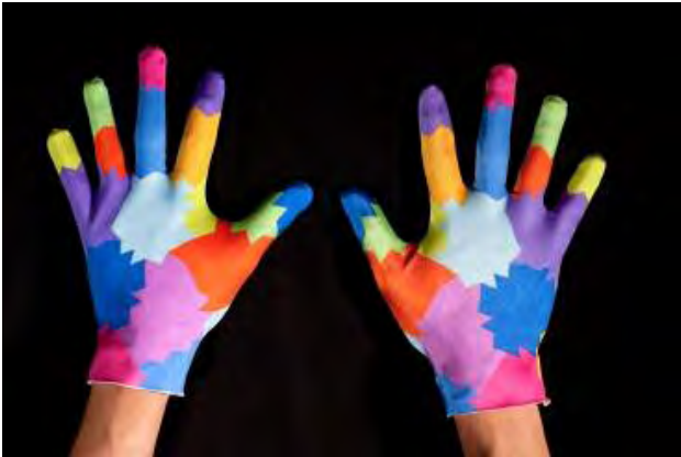
The hardware for a new gesture-based computing system consists of nothing more than an ordinary webcam and a pair of brightly colored lycra gloves. Photo: Jason Dorfman/CSAIL
