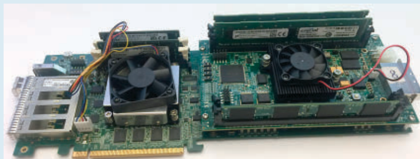
Figure 5. A prototype programmable SSD developed for research purposes.
