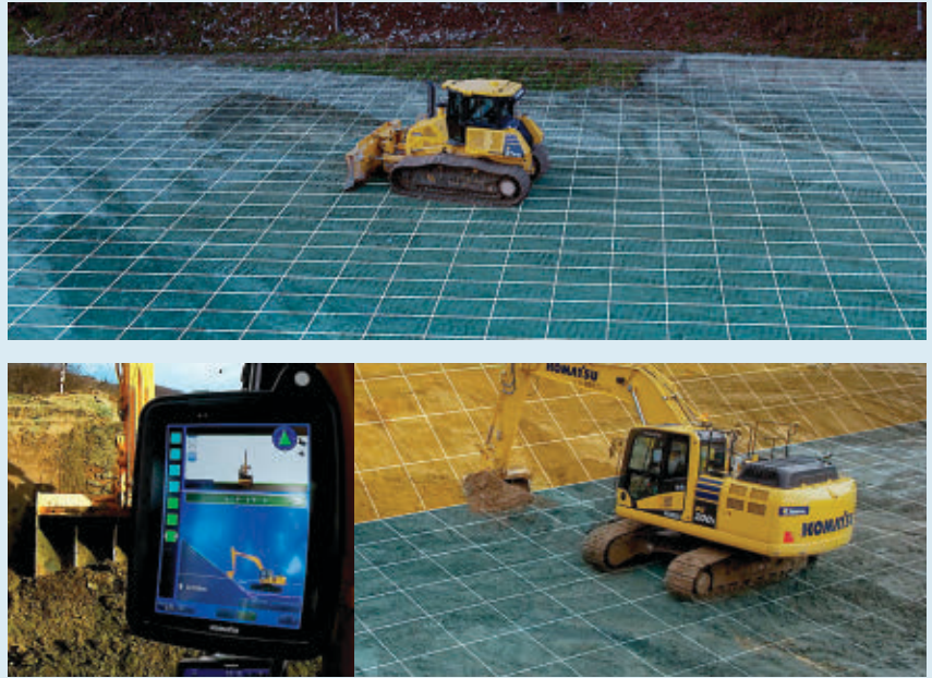
Komatsu excavator uses computation to calculate the correct angle of its digging blade.
