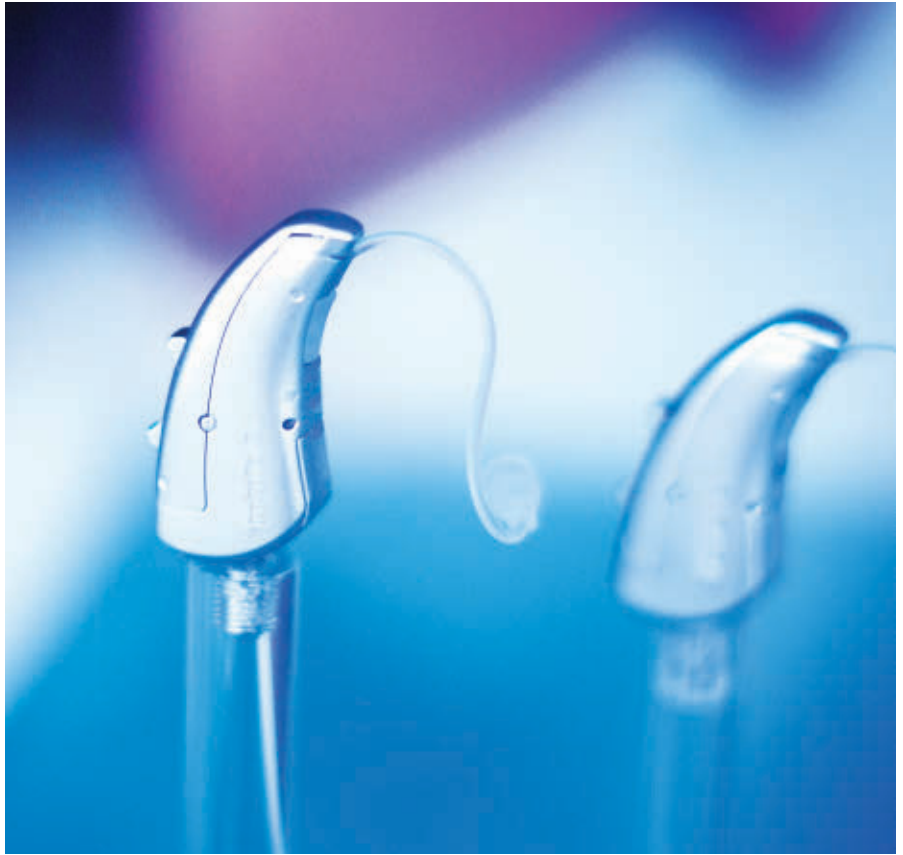
The Earlens Light-Driven Hearing Aid converts sounds into pulses of light, which activate a lens on the eardrum.
