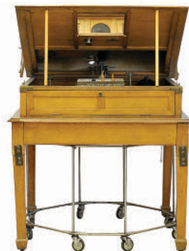
Figure 11. Second automatic chess endgame machine by Torres Quevedo, playing with king and rook (automaton) vs. king (human player). Courtesy of Museo Leonardo Torres Quevedo, Universidad Politécnica de Madrid, Spain.
