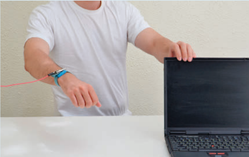
Figure 2. Measuring the chassis potential by touching a conductive part of the laptop; the wristband is connected to signal-acquisition equipment.
