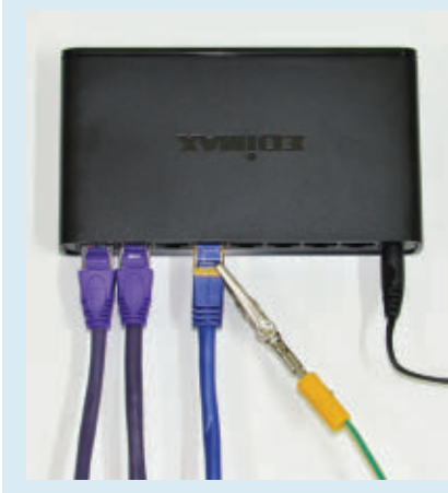
Figure 7. Measuring the chassis potential from the far side of an Ethernet cable (blue) plugged into the target laptop (10 meters away) through an alligator clip leading to measurement equipment (green wire).
