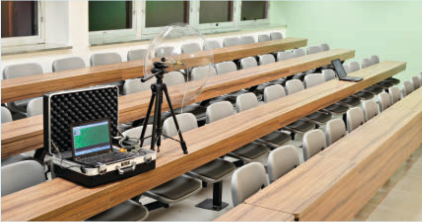
Figure 1. An acoustic attack using a parabolic microphone (left) on a target laptop (right); keys can be extracted from a distance of 10 meters.
