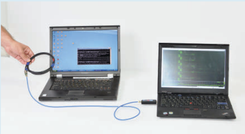
Figure 9. Measuring electromagnetic emanations from a target laptop (left) through a loop of coax cable (handheld) recorded by a software-defined radio (right).
