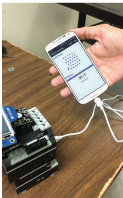
A prototype of a portable assay device connected to a smartphone; such equipment could help remote farmers diagnose crop diseases without access to a full lab.
