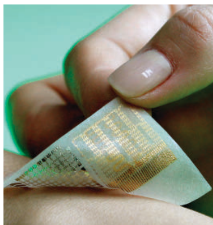
This prototype electronic skin patch can store and transmit data about a person's movements, receive diagnostic information, and release drugs into skin.
