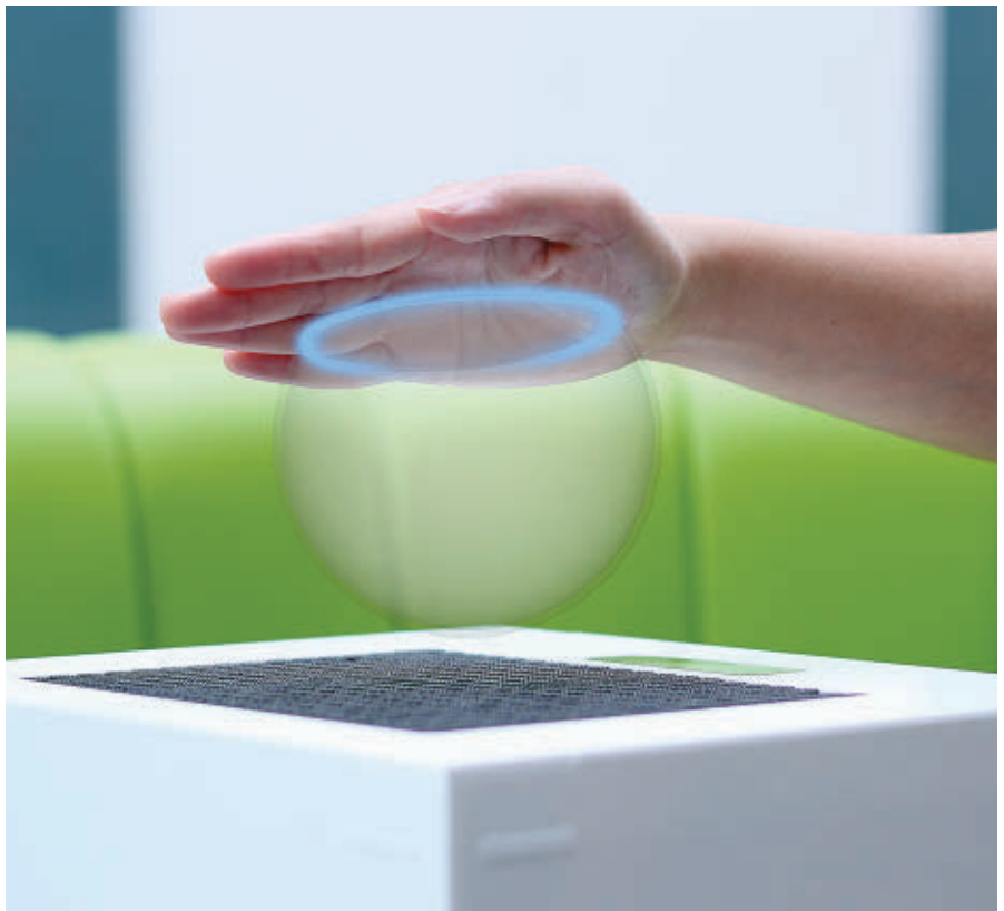
Ultrasound is focused to create the shape of a virtual sphere that may be felt.
