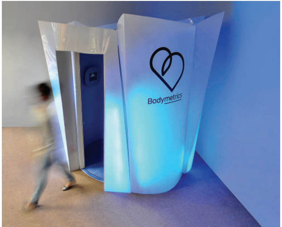
As many as 200 of a woman's measurements are captured by 16 Kinect devices inside a Bodymetrics walk-in pod, in order to generate a 3D body scan that can be used to match her physical attributes to specific articles of clothing.
