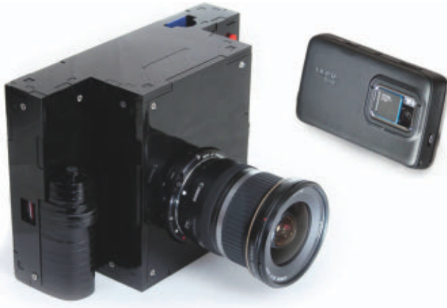
Figure 1. Two implementations of the Frankencamera architecture: The custom-built F2 (left)—portable and self-powered, best for projects requiring flexible hardware; and the Nokia N900 (right) with a modified software stack—a compact commodity platform best for rapid development and deployment of applications to a large audience.
