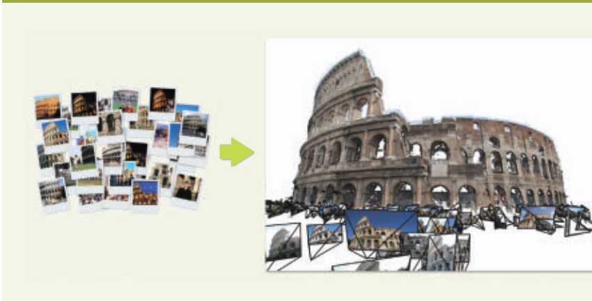
Figure 3. 3D model of a scene (right) generated from photographs (left).
