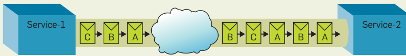
Figure 4. In most loosely coupled systems, messages may arrive multiple times and out of order.
