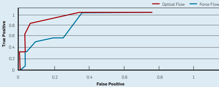
Figure 9. ROC curves for detection of abnormal behaviors in the University of Minnesota data set; the area under the social force curve (red) is 0.96, and the area under the optical flow curve (blue) is 0.84.
