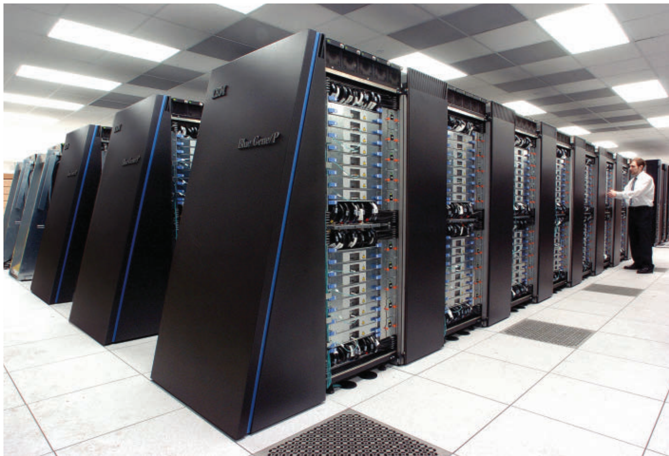
Figure 1. The Intrepid Blue Gene/P Open Science machine at Argonne National Laboratory, with 163,840 cores and 557TFlops/sec (peak).
