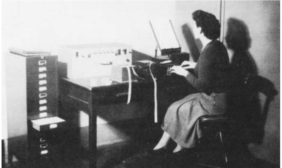
The EDSAC subroutine library was kept in the steel cabinet on the left in the image. Library tapes were copied mechanically onto the user's program tape and then returned to the cabinet.
