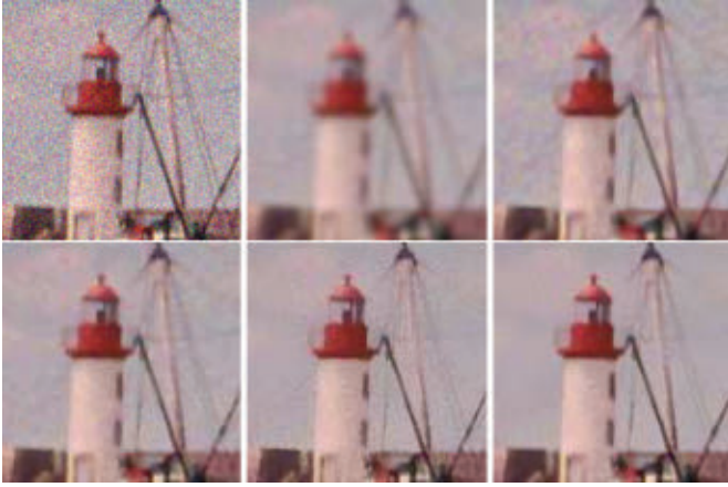
Figure 7. Denoising experience on a natural image. From left to right and from top to bottom: noisy image (standard deviation \sigma = 20 ), Gaussian convolution ( h = 1.8 ), anisotropic filter ( h = 2.4 ), total variation ( \lambda = 0.04 ), the Yaroslavsky neighborhood filter ( \rho = 7 , h = 28 ), and the NL-means algorithm. Parameters have been set for each algorithm so that the removed quadratic energy is equal to the energy of the added noise.
