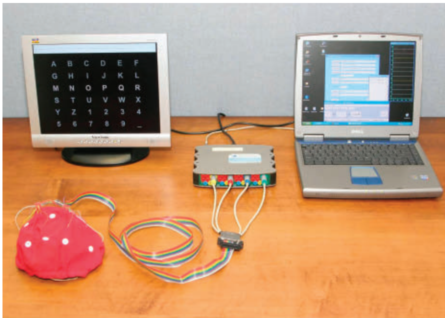
Figure 5. Hardware in the Wadsworth Center's home BCI system, including 16-channel electrode cap for signal recording, solid-state amplifier, laptop, and additional monitor as user display.
