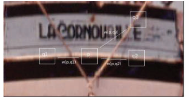
Figure 2. q1 and q2 have a large weight in NL-means because their similarity windows are similar to that of p, while the weight w(p, q3) is much smaller.
