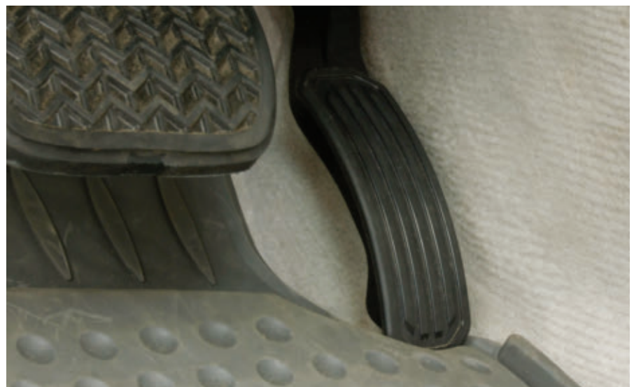
Example of an unsecured driver-side floor mat trapping the accelerator pedal in a 2007 Lexus ES350.
